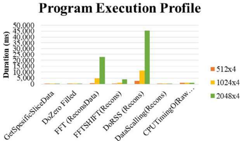
FIGURE 4. Program Execution profile. The hotspot of the MRI Image Reconstruction energy consumption is in DoRSS Function
