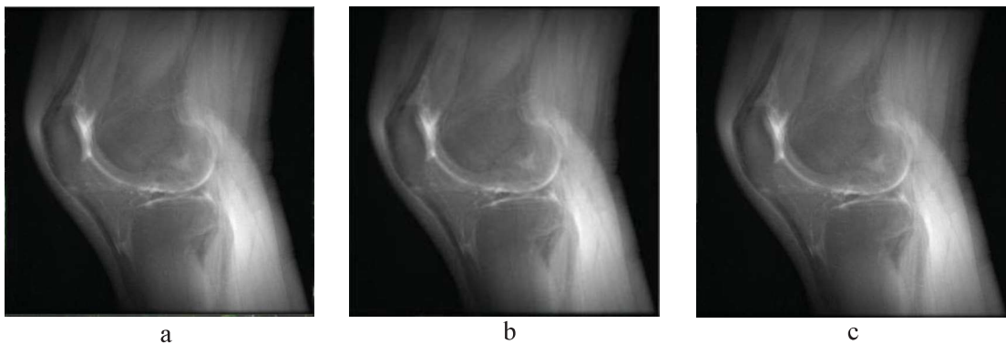
FIGURE 2. MRI Image reconstructed through inverse FFT with Zero Filling. (a) Image by 512x512 inverse FFT, (b) Image by 1024x1024 inverse FFT, (c) Image by 2048x2048 Inverse FFT
